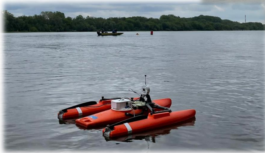
Over 1.5h of operation on one battery pack
