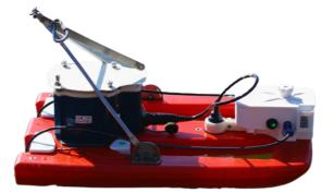
Stork Remote System (SRS) has been designed to allow TRDI StreamPro ADCP users to perform discharge measurements in streams, rivers and lakes easier and faster, without even entering the water. Easy to mount, plug&play set of two thrusters, battery package and R/C controller. Changing your standard tethered float into Unmanned Surface Vessel (USV) will take only few minutes.
